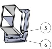
Install the supplied #10 x 1" stainless steel snap cap screw in the hole on the side of the bracket. Make sure it goes into the aluminum or galvanized stiffener.
