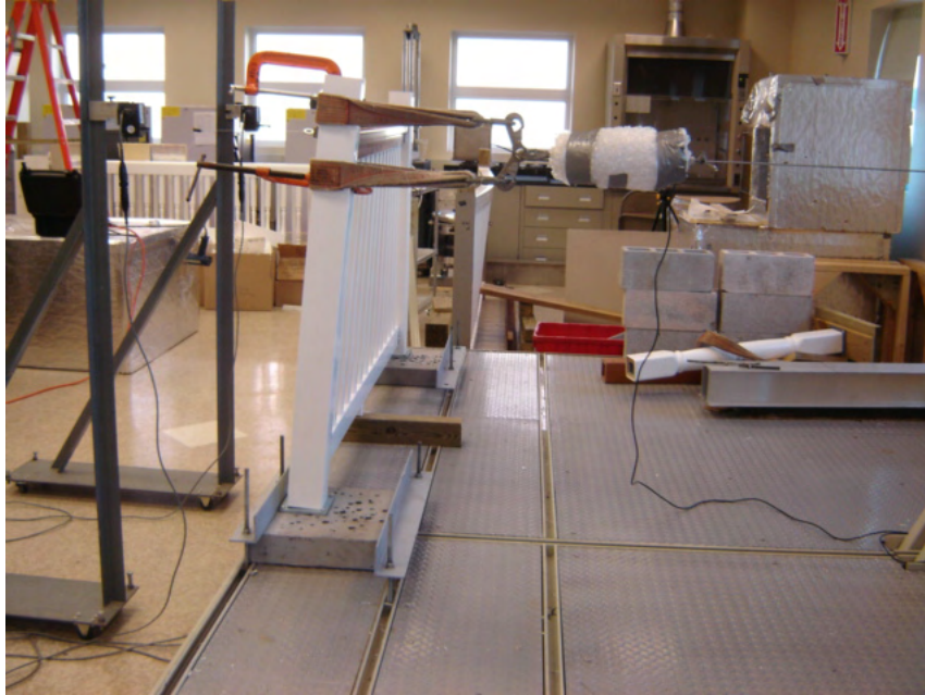
Photo No. 7 Concentrated Load at Top of Post
