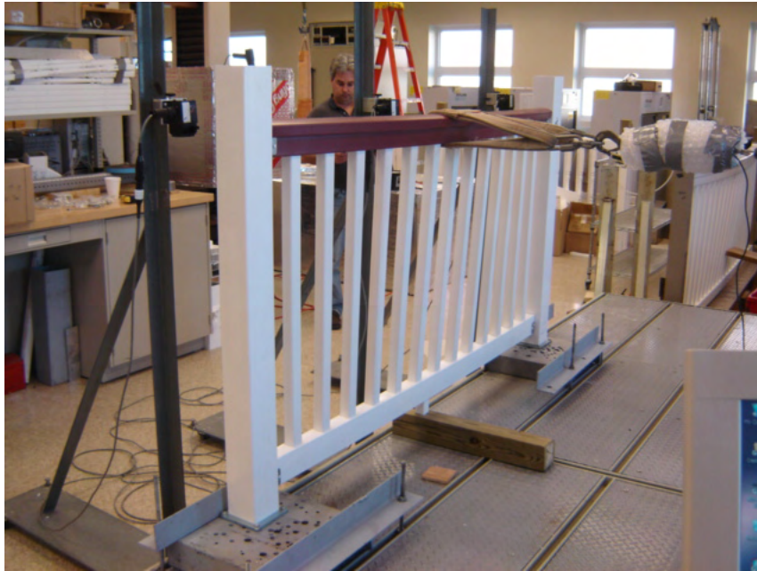
Photo No. 5 Concentrated Load at Midspan of Top Rail
