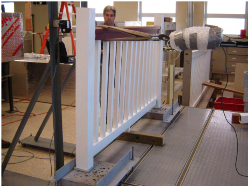
Photo No. 6 Concentrated Load at End of Top Rail (Bracket)
