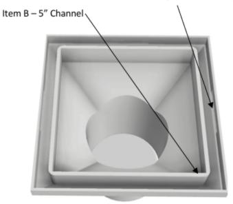
Insert the interior 5" channel into the 5" vinyl post by angling it slightly and pressing it firmly into place.
