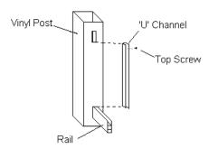
Next set end posts and corner posts at desired height by inserting another screw through the 'u' channel into the collars. Then by running a string over top and between the end and corner posts you can set the rest of the posts to height by lifting to string and fastening through 'u' channel to the collars...
