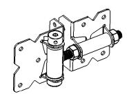
The hinges should be inspected annually or more frequently if the gate is used often. Spring tension adjustments should be made as needed. If needed, the spring can be lubricated with an oil based lubricant applied to the cam and barrel portion of the hinge.
