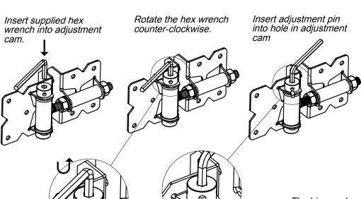
Carefully rotate the adjustment cam clockwise until the adjustment pin contacts the fence post leaf. Remove the hex wrench. Repeat until gate closes firmly.
